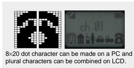
8x20 dot character can be made on a PC and plural characters can be combined on LCD.
